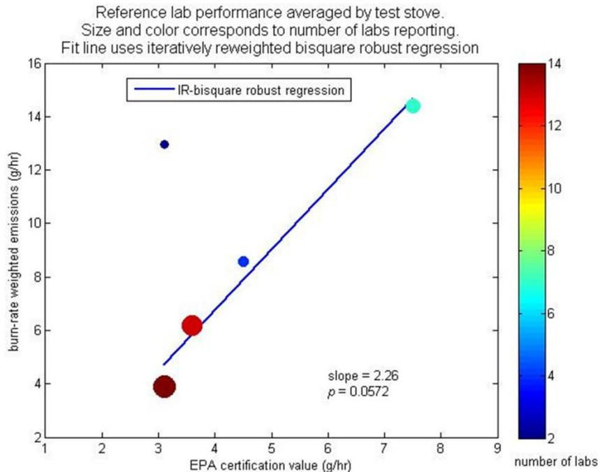
**Figure 1.** Robust regression of round robin testing data from EPA certified reference stoves. The size and color of the dots indicates the number of lab reports.
