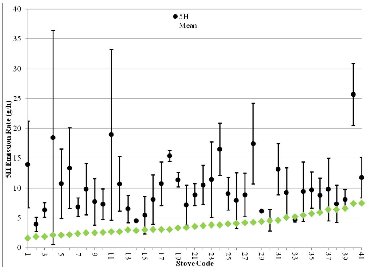
Figure 14. Mean Emission Rates, Standard Deviations around Means, and EPA Certification Values by Stove Model
