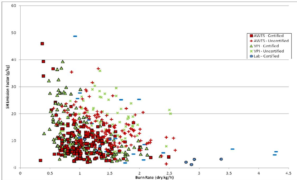
Figure ES6. Emission Rates (top) and Emission Factors (bottom) versus Burn Rates for All Stove Tests. (“Lab” refers to tests conducted in the laboratory using consumer burn practices not EPA Method 28.)
