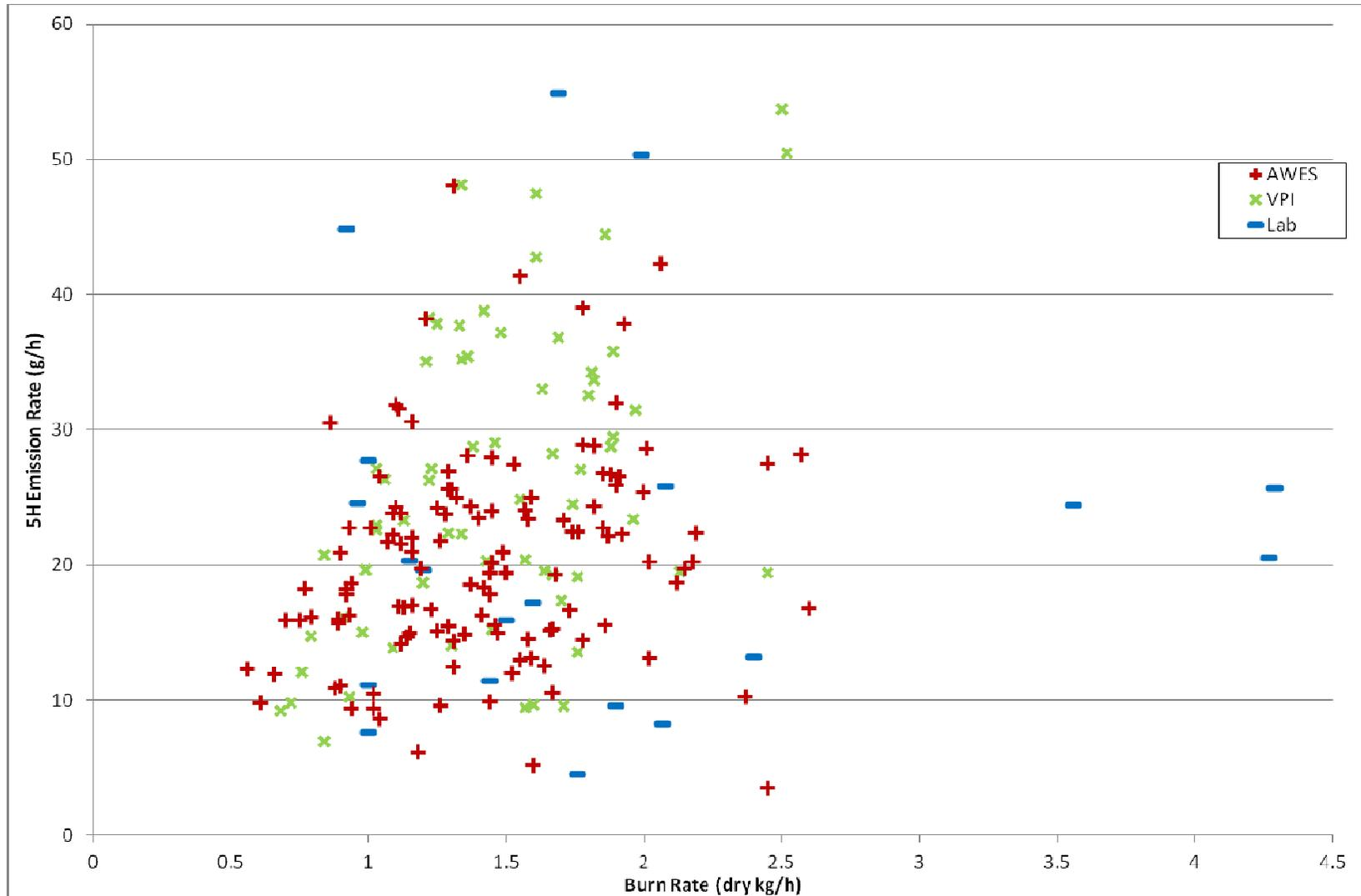
Figure 4. Emission Rates by Test Run versus Burn Rates – Uncertified Stoves Only. (Burn rate data are as reported in the various in-home AWES studies, in-home VPI studies, and laboratory studies that simulate in-home usage with cordwood. They are not as described in 40CFR Part 60 Appendix A Method 28 for certification.)
