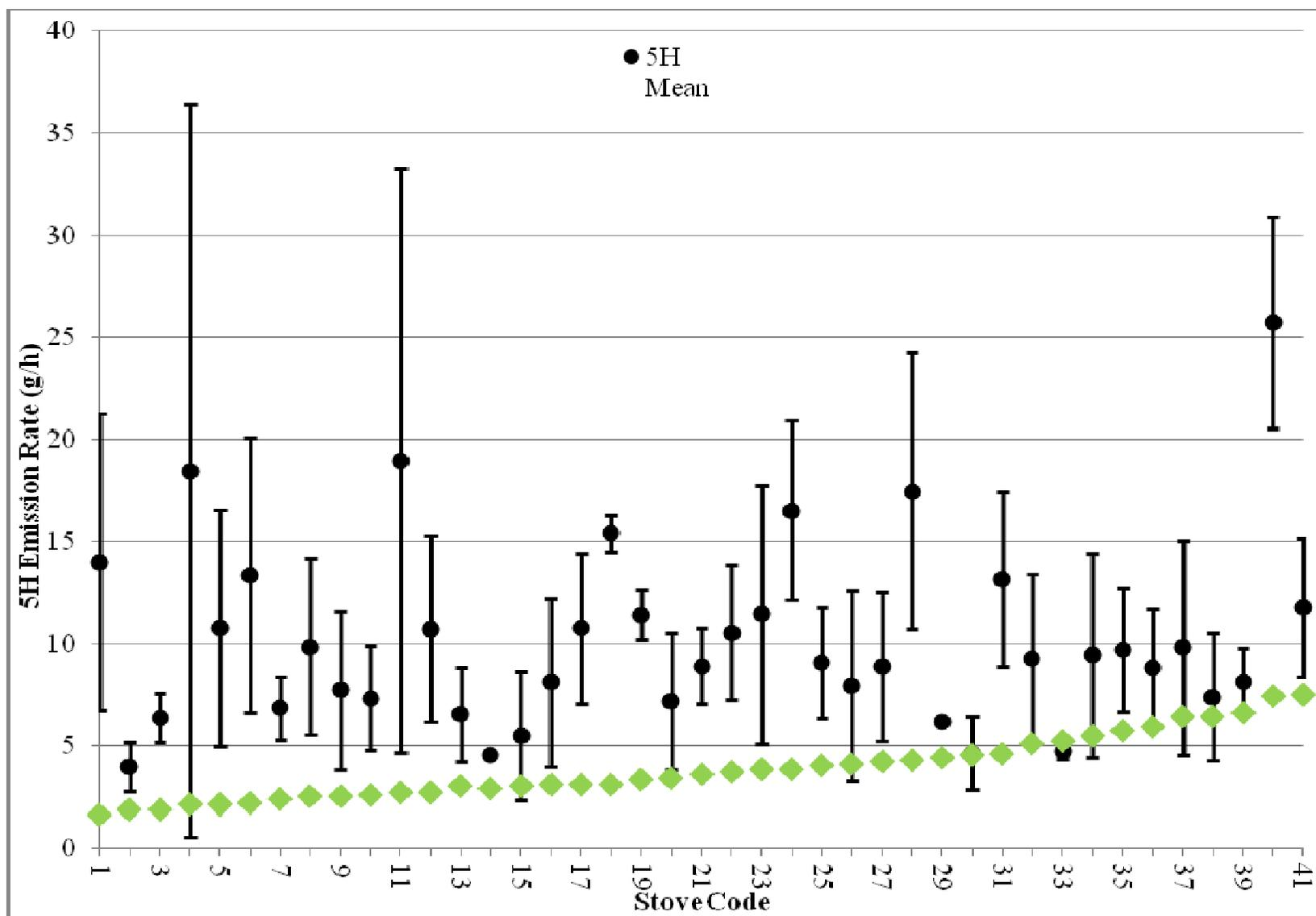
Figure ES2. Mean Emission Rates, Standard Deviations around Means, and EPA Certification Values by Stove Model. (Each stove model was assigned a stove code.)
