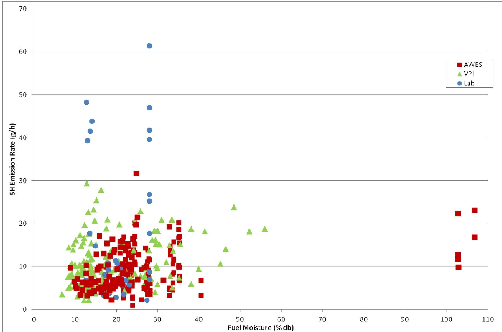
Figure 8. Emission Rates by Test Run versus Wood Moistures – Certified Stoves Only. (“Lab” refers to tests conducted in the laboratory using consumer burn practices not EPA Method 28.)
