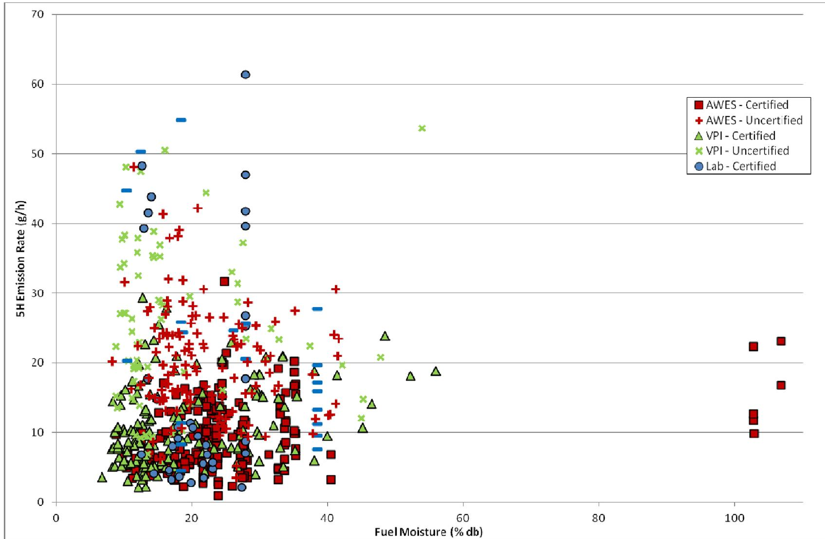
Figure12. Emission Rates by Test Run versus Wood Moistures – All Stoves. (“Lab” refers to tests conducted in the laboratory using consumer burn practices not EPA Method 28.)
