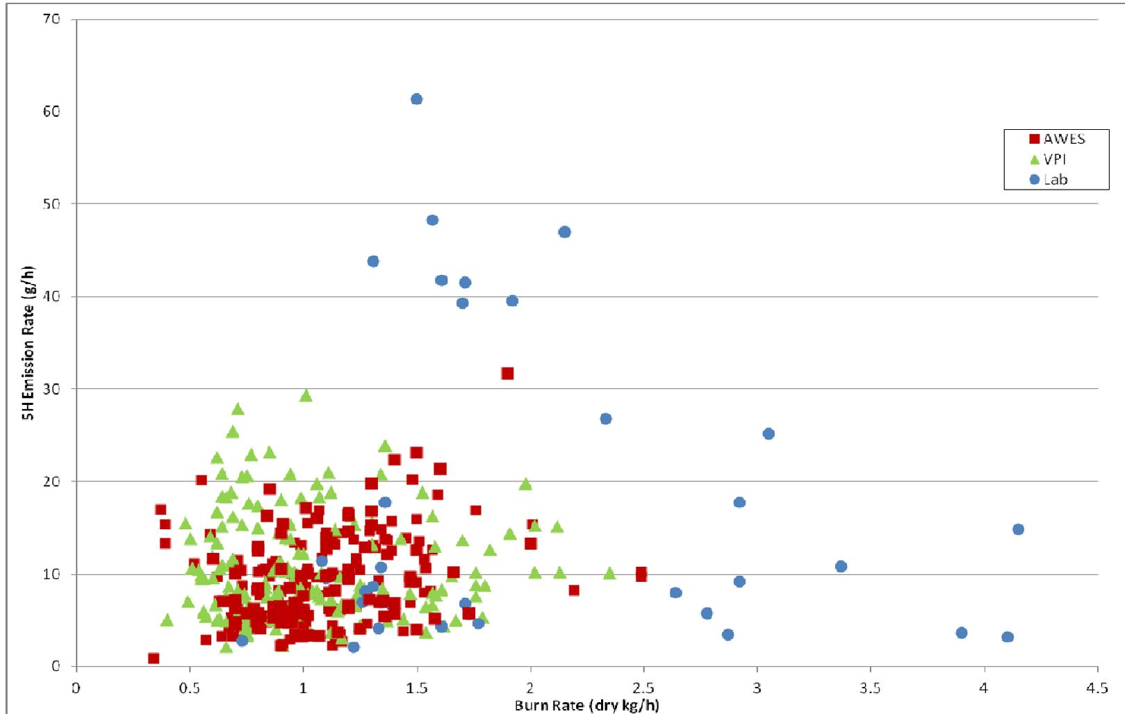
Figure 2. Emission Rates by Test Run versus Burn Rates – Certified Stoves Only. (Burn rate data are as reported in the various in-home AWES studies, in-home VPI studies, and laboratory studies that simulate in-home usage with cordwood. They are not as described in 40CFR Part 60 Appendix A Method 28 for certification.)
