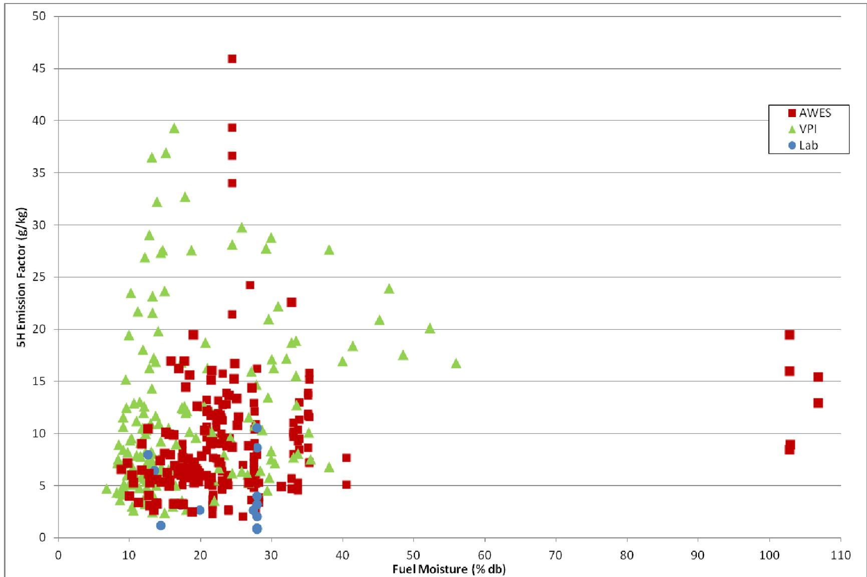
Figure 9. Emission Factors by Test Run versus Wood Moistures – Certified Stoves Only. (“Lab” refers to tests conducted in the laboratory using consumer burn practices not EPA Method 28.)
