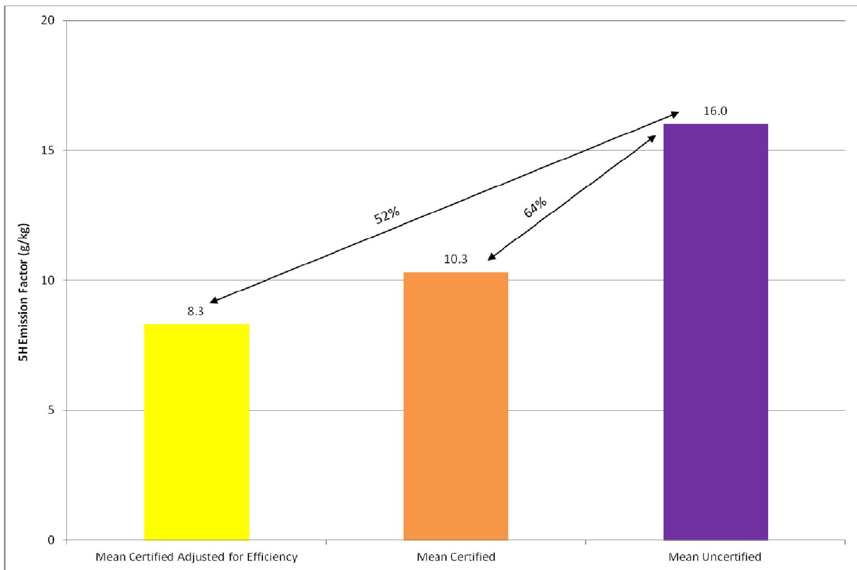
Figure ES5. Comparison of the Mean Effective Emission Factor of Certified Cordwood Stoves (Adjusted for Efficiency) with the Mean Emission Factor of Uncertified Stoves. The mean of all certified emission factors adjusted for efficiency is 52% of the mean of all uncertified emission factors ( $8.3/16.0 \times 100\%$ ).
