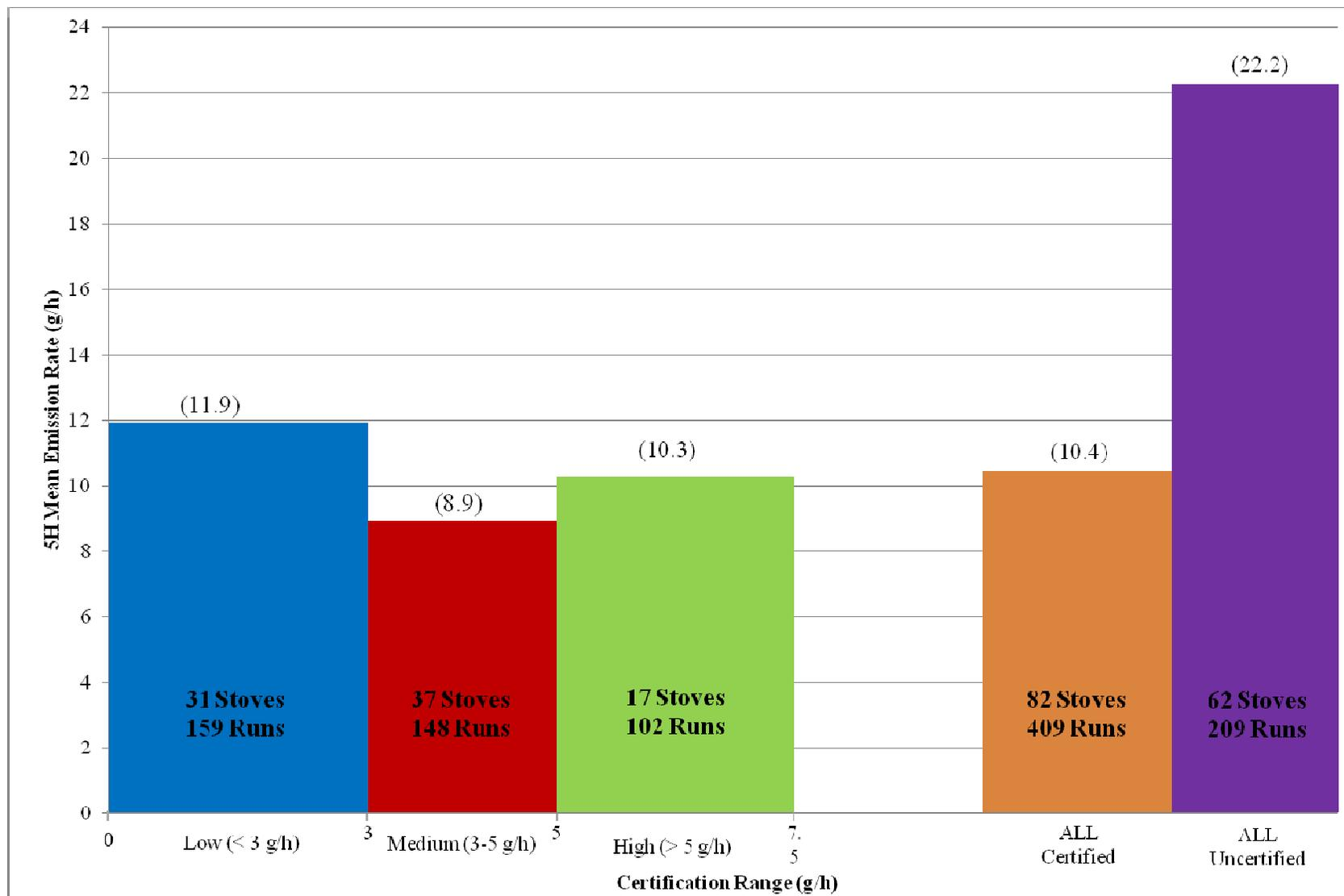
Figure ES3. Mean Emission Rates for Uncertified Stoves and for Certified Stoves by Low, Medium, and High Certification Categories. The mean of all certified emission rates is 47% of the mean of all uncertified emission rates (10.4/22.2 X 100%).
