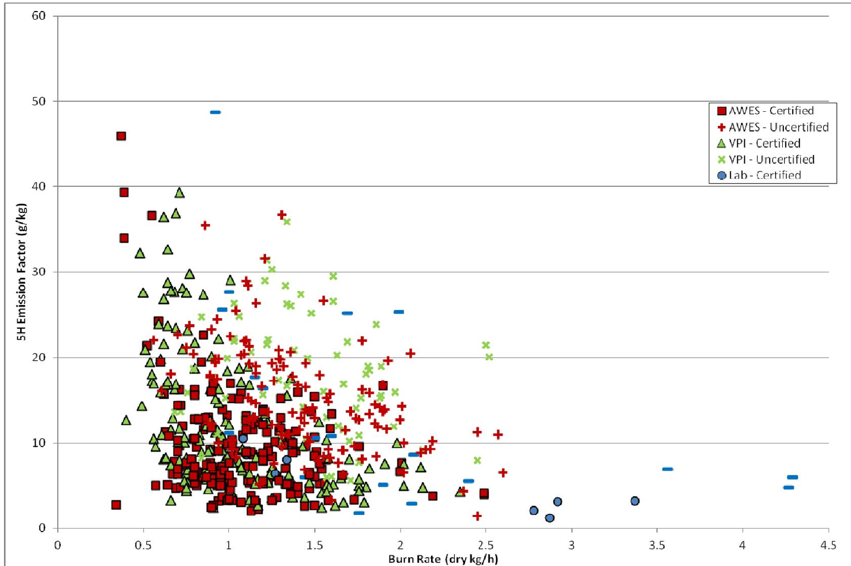
Figure 7. Emission Factors by Test Run versus Burn Rates – All Stoves. (Burn rate data are as reported in the various in-home AWES studies, in-home VPI studies, and laboratory studies that simulate in-home usage with cordwood. They are not as described in 40CFR Part 60 Appendix A Method 28 for certification.)
