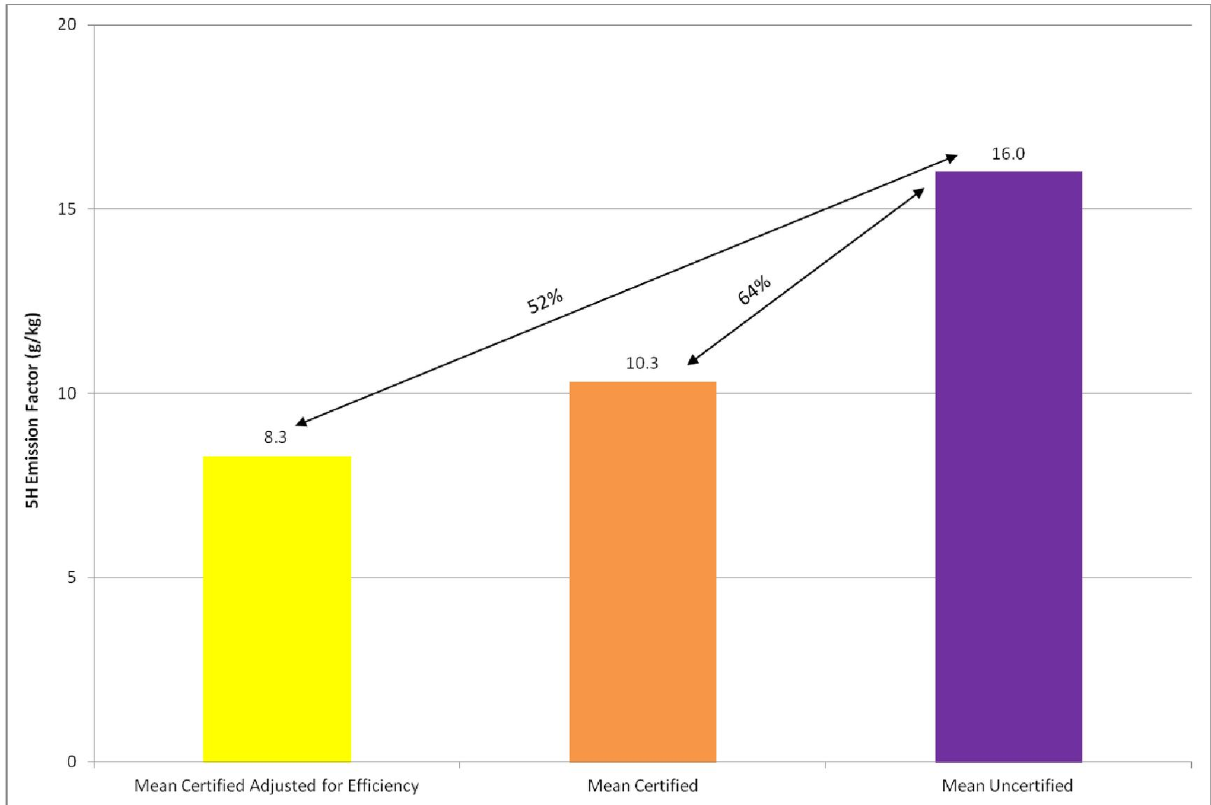
Figure19. Comparison of the Mean Effective Emission Factor of Certified Cordwood Stoves (Adjusted for Efficiency) with the Mean Emission Factor of Uncertified Stoves
