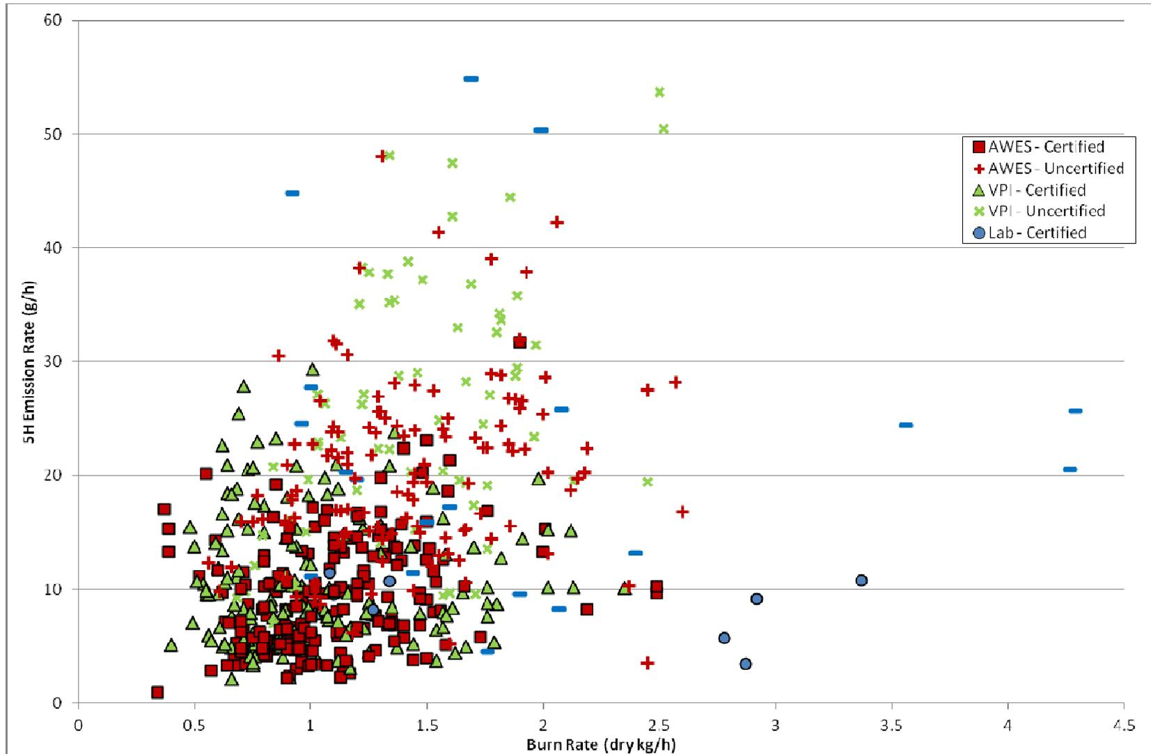
Figure 6. Emission Rates by Test Run versus Burn Rates – All Stoves. (Burn rate data are as reported in the various in-home AWES studies, in-home VPI studies, and laboratory studies that simulate in-home usage with cordwood. They are not as described in 40CFR Part 60 Appendix A Method 28 for certification.)
