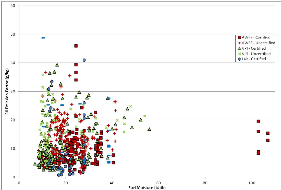
Figure ES7. Emission Rates (top) and Emission Factors (bottom) versus Wood Moisture for All Stove Tests. (“Lab” refers to tests conducted in the laboratory using consumer burn practices not EPA Method 28.)
