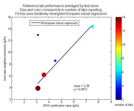
**Figure 1.** Robust regression of round robin testing data from EPA certified reference stoves. The size and color of the dots indicates the number of lab reports.
