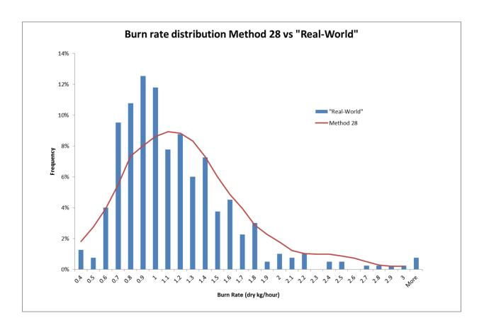
**Figure 6.** Burn rate histogram of all test data (bars) and the distribution specified by Method 28. The "real-world" data shows substantially more data collected from stoves operating at burn rates of 0.7-1.0 kg/hour than is specified by EPA certification Method 28. Considering the bi-modal behavior of some stoves, and the great sensitivity of their emissions rates on the burn rate, this burn rate inconsistency is likely to have introduced, or reflect a substantial bias
