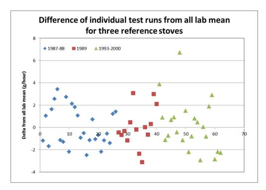
**Figure 2**. Residuals of the individual tests runs from the mean of all tests for that individual stove. The standard deviation is 1.8 g/hour. Three two-way Kolmogorov-Smirnov tests showed no significant difference between these sets of residuals (*p*>0.38).
