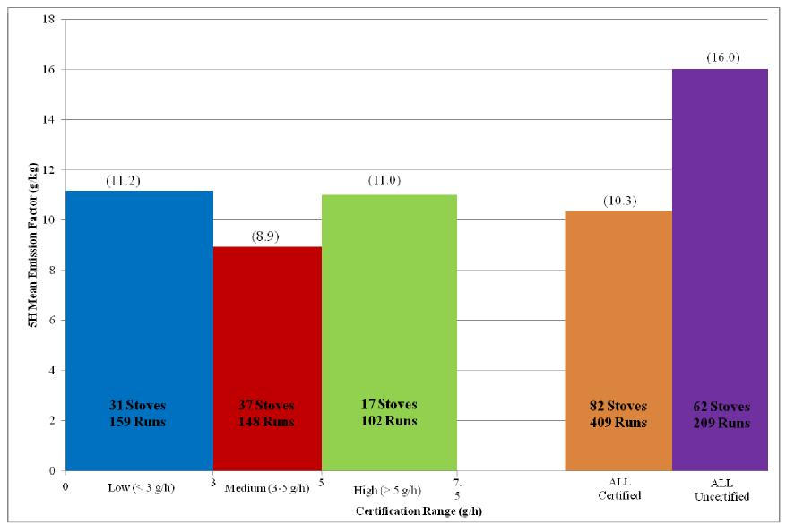
Figure ES4. Mean Emission Factors for Uncertified Stoves and for Certified Stoves by Low, Medium, and High Certification Categories. The mean of all certified emission factors is 64% of the mean of all uncertified emission factors (10.3/16.0 X 100%).
