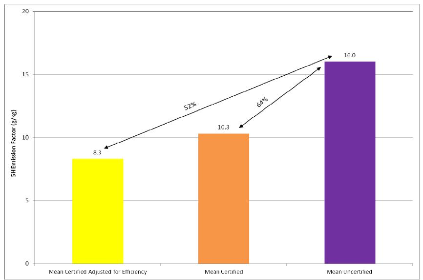
Figure ES5. Comparison of the Mean Effective Emission Factor of Certified Cordwood Stoves (Adjusted for Efficiency) with the Mean Emission Factor of Uncertified Stoves. The mean of all certified emission factors adjusted for efficiency is 52% of the mean of all uncertified emission factors (8.3/16.0 X 100%).
