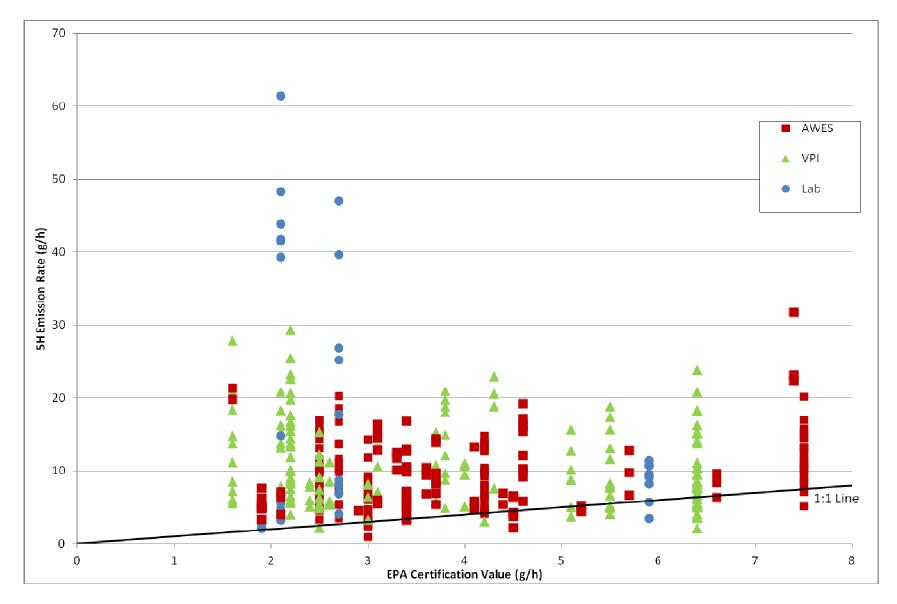
Figure 1. Emission Rates by Test Run versus EPA Certification Values for Stove Models. ("Lab" refers to tests conducted in the laboratory using consumer burn practices not EPA Method 28.)
