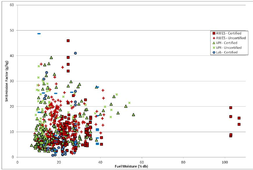
Figure 13. Emission Factors by Test Run versus Wood Moistures – All Stoves. ("Lab" refers to tests conducted in the laboratory using consumer burn practices not EPA Method 28.)
