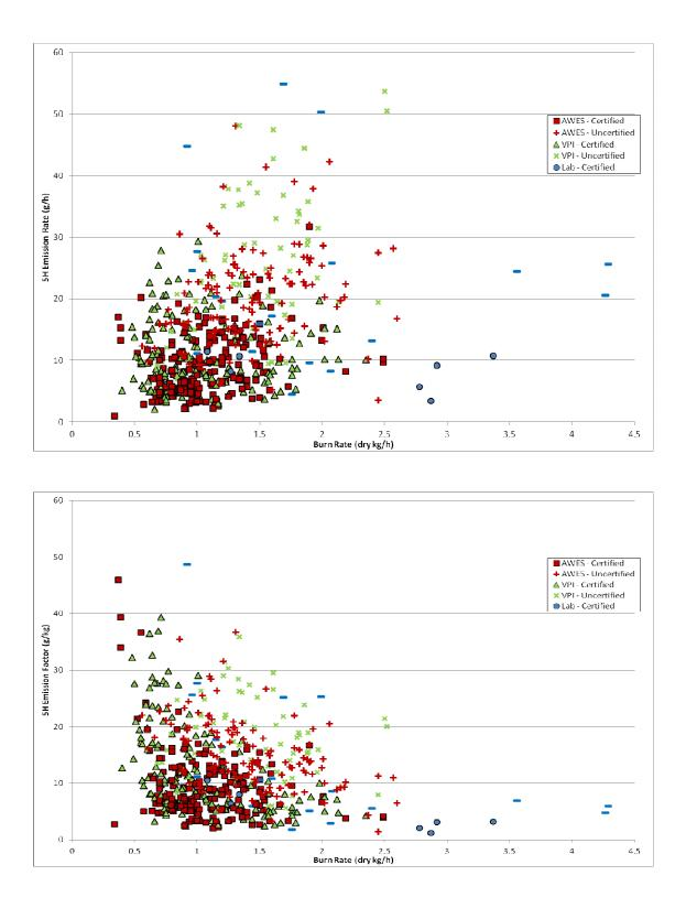
Figure ES6. Emision Rates (top) and Emission Factors (bottom) versus Burn Rates for All Stove Tests. ("Lab" refers to tests conducted in the laboratory using consumer burn practices not EPA Method 28.)
