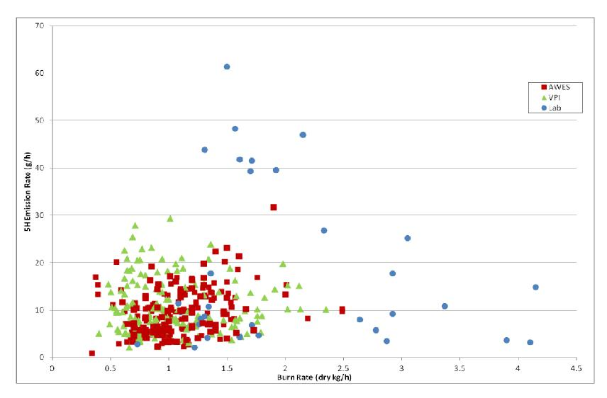
Figure 2. Emission Rates by Test Run versus Burn Rates – Certified Stoves Only. (Burn rate data are as reported in the various inhome AWES studies, in-home VPI studies, and laboratory studies that simulate in-home usage with cordwood. They are not as described in 40CFR Part 60 Appendix A Method 28 for certification.)
