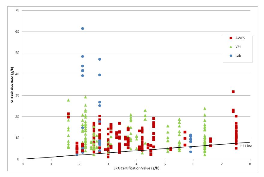
Figure ES1. Emission Rates by Test Run versus EPA Certification Values for Stove Models . ("Lab" refers to tests conducted in the laboratory using consumer burn practices not EPA Method 28.)
