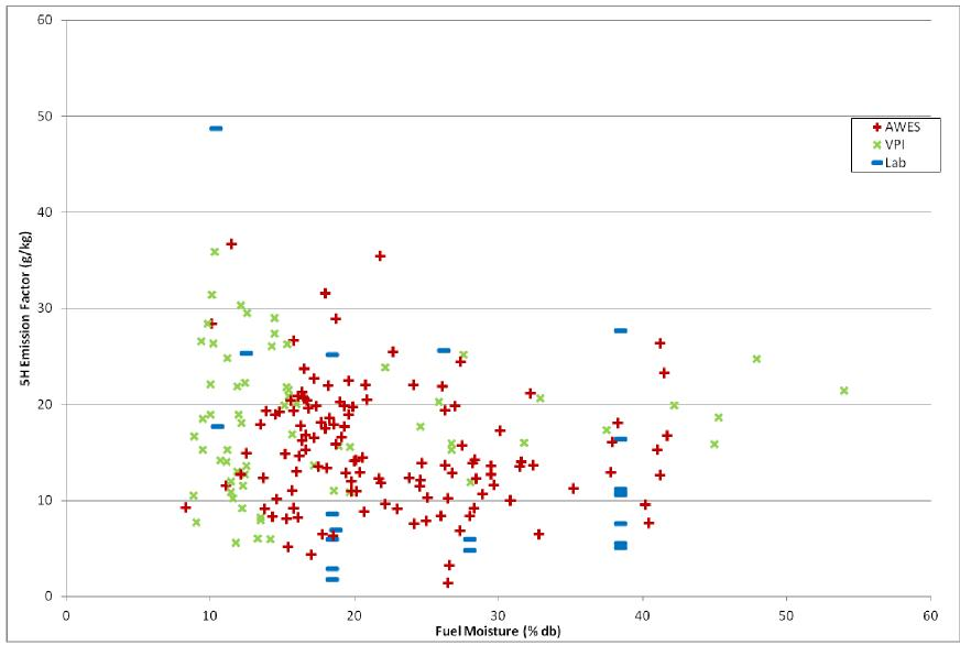
Figure 11. Emission Factors by Test Run versus Wood Moistures – Uncertified Stoves Only. ("Lab" refers to tests conducted in the laboratory using consumer burn practices not EPA Method 28.)
