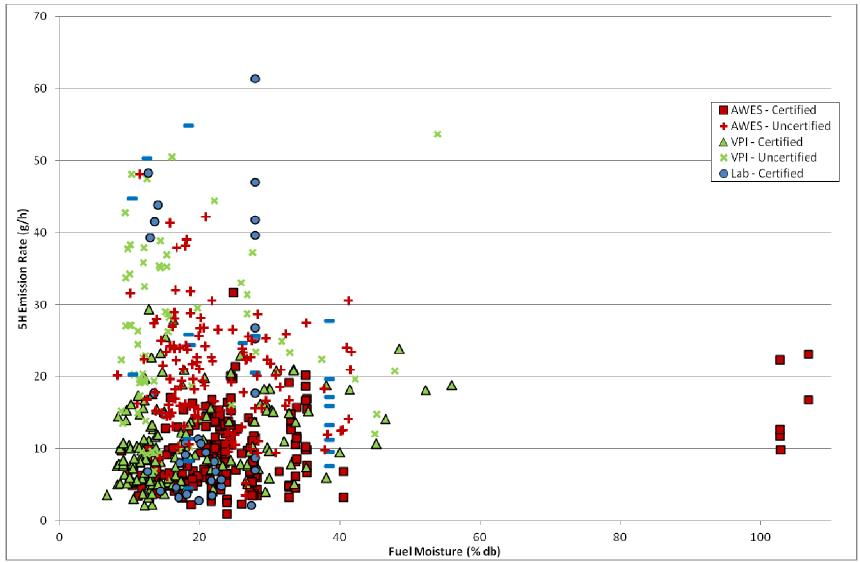
Figure 12. Emission Rates by Test Run versus Wood Moistures – All Stoves. ("Lab" refers to tests conducted in the laboratory using consumer burn practices not EPA Method 28.)
