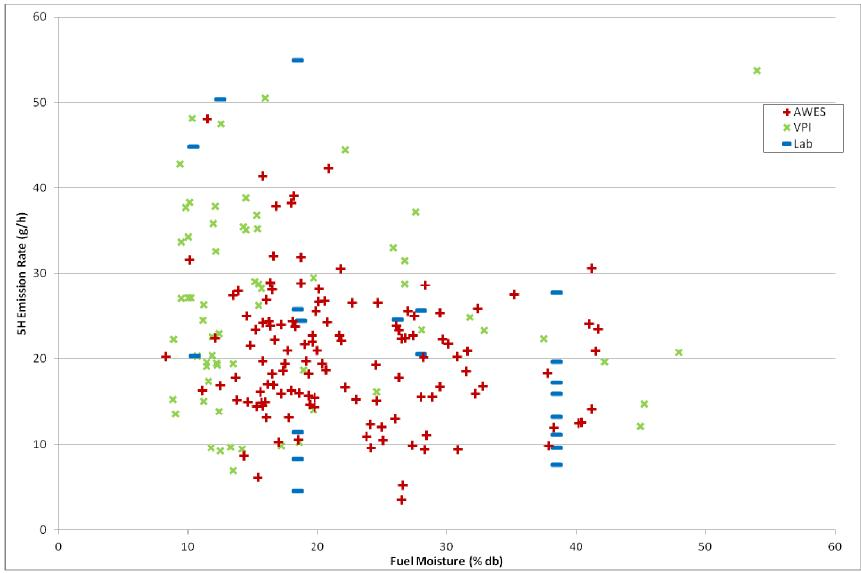
Figure 10. Emission Rates by Test Run versus Wood Moistures – Uncertified Stoves Only. ("Lab" refers to tests conducted in the laboratory using consumer burn practices not EPA Method 28.)
