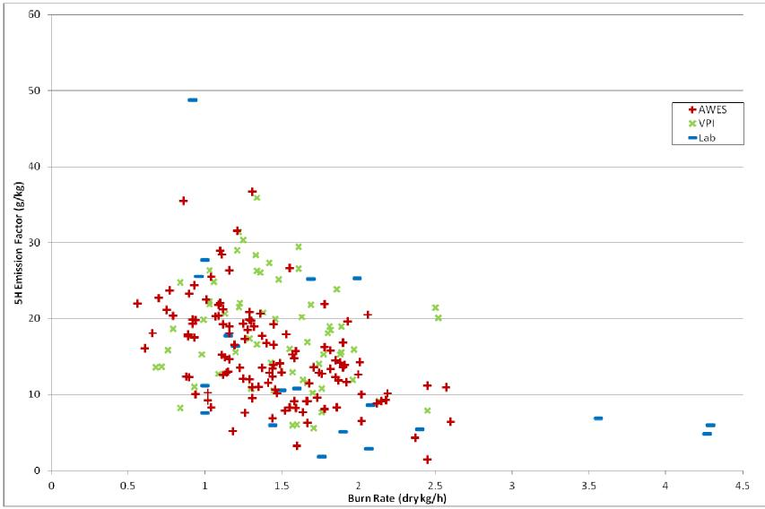
Figure 5. Emission Factors by Test Run versus Burn Rates – Uncertified Stoves Only. (Burn rate data are as reported in the various in-home AWES studies, in-home VPI studies, and laboratory studies that simulate in-home usage with cordwood. They are not as described in 40CFR Part 60 Appendix A Method 28 for certification.)
