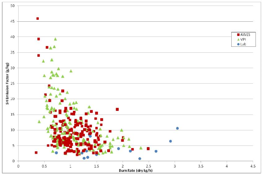
Figure 3. Emission Factors by Test Run versus Burn Rates – Certified Stoves Only. (Burn rate data are as reported in the various inhome AWES studies, in-home VPI studies, and laboratory studies that simulate in-home usage with cordwood. They are not as described in 40CFR Part 60 Appendix A Method 28 for certification.)
